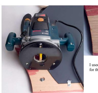
I used a router to provide the recessed area for the bolt heads and nuts.
