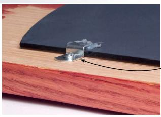
The mirror clips are used to hold the mirror. I purchased them at a local home improvement center. The mirror clips are actually for a thicker piece of glass so I used silicone to fill the gap.
