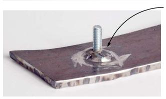
The head of the bolt was welded to the steel plate. This resulted in a large area that will project into the oak wood. You will need to use a router to provide a
